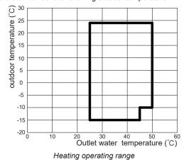
c. Model 130kW&260kW: The unit is of outlet water temperature control mode
