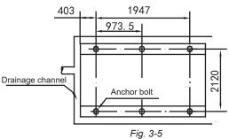
Schematic diagram of installation dimension of Model 260kW.
