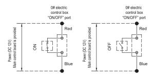
If the "ON/OFF" port is effective ,the "Net on" icon of the wire controller will be flashing.
