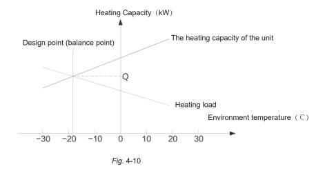
If the design point and the balance point do not coincide, the heating capacity of the unit at the design point (Q2) will be less than the building heat load (Q1). In this case, electric heating must be configured with a power output equal to the difference between Q1 and Q2.
