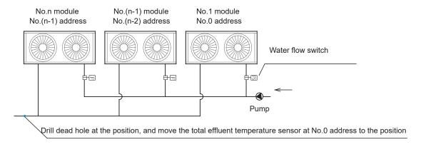
Fig. 4-8 130 model (Only 16 modular units can be combined at most)
