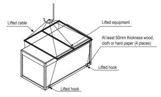
Fig. 2-1 Lifting of the unit
