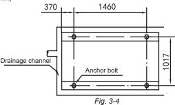
Schematic diagram of installation dimension of Model 130kW.
