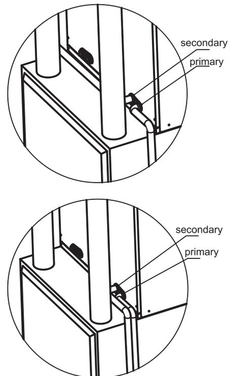
Fig. 4-2 DRAIN PIPE ROUTING
