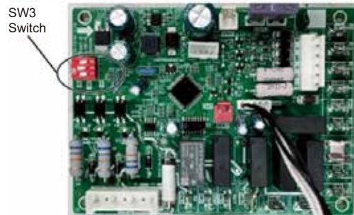
Fig.7 SW3 Switch Location in the PCB Board (For reference only)
