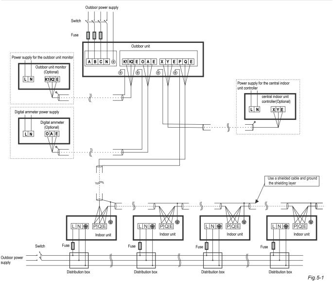
200/224/260 Three-phase electrical control system connection of the outdoor unit
