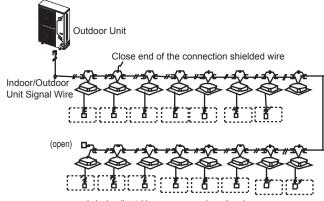
In broken line table, users can purchase the wire controller when necessary.
